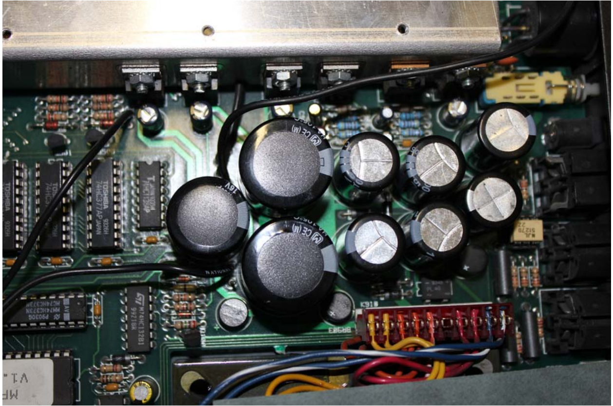
When finished it should look like this. Pay attention to the polarity of the caps!!!!!!
